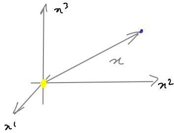
$$\begin{aligned} \mathbf{r} &= \begin{pmatrix} x^1 \\ x^2 \\ x^3 \end{pmatrix} \\ r &= \sqrt{(x^1)^2 + (x^2)^2 + (x^3)^2} \end{aligned}$$
